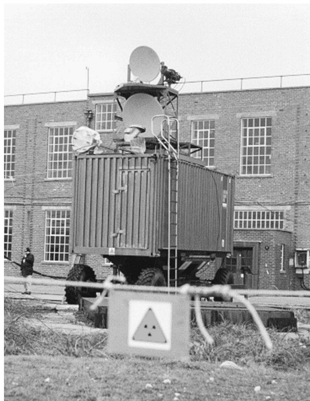
FIG. 21. Photograph of a nanosecond radar system. (Reproduced with the permission of GEC-Marconi and the United Kingdom Ministry of Defense.)
