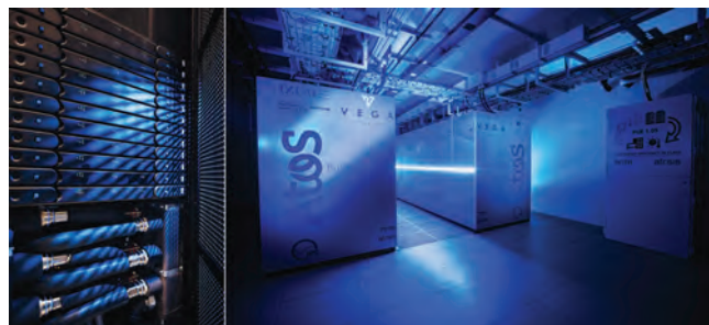
Figure 3: Located at IZUM, the new Slovenian supercomputer Vega was designed and set-up with support of JSI experts. The new system with close to 6.8 peta FLOP/s of raw computing power, 20 PB of storage and broadband connectivity has put Slovenia in 21st place in the November's Top500 list of supercomputing capacity per number of inhabitants.
