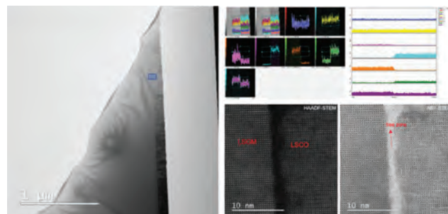
Figure 13: HAADF STEM and ABF STEM images of the free zone in the LSCO/(100)LSGM thin film (Sandra Drev, CEMM, JEM-ARM200F)
