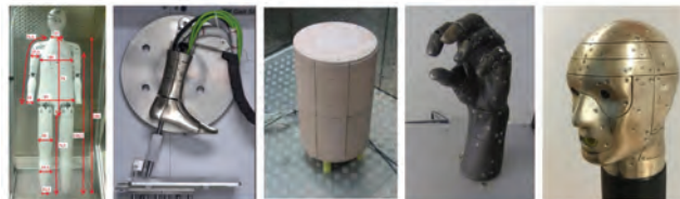
Figure 7: Sweating thermal manikins for testing protective garments
