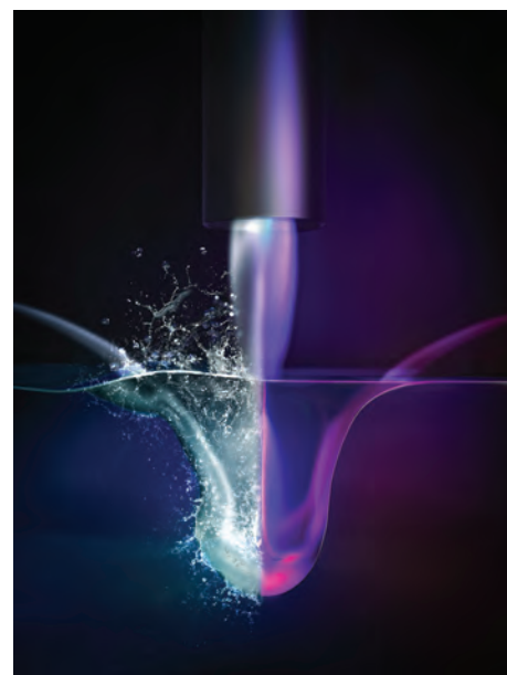
Figure 1: Cavity (or dimple) formation at the water surfaces subjected to a neutral helium-gas jet (left) and a weakly ionized helium-gas jet (right)
