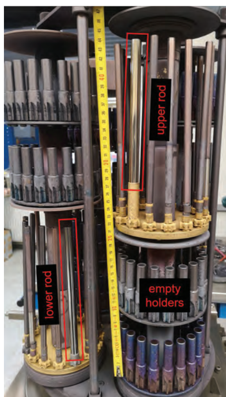
Figure 3: Case of a test batch construction in the industrial deposition chamber; we applied polished high-speed steel rods for the continuous vertical evaluation of the coating properties.
