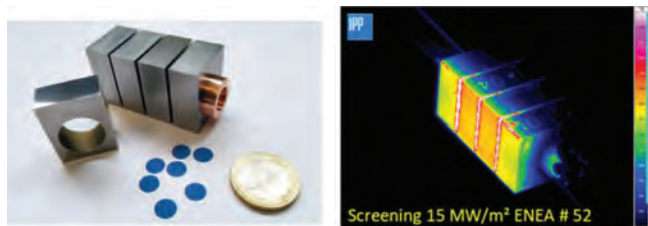
Figure 10: W-11WC monoblock joint with a CuCrZr tube (left); the same mock-up exposed to a thermal shock of 15 MW/m 2 while being cooled with a cooling liquid (at a temperature of 18 °C) (right)
