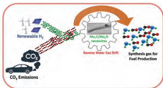
Figure 5: The global carbon footprint can be mitigated by utilizing the renewable nature of CO 2 , where it could be captured, stored, and used for the production of various fuels through carbon capture and utilization technology. A highly promising path is a direct Fischer-Tropsch type process in one reactor with a reverse water gas shift reaction (RWGS) using carbon dioxide in combination with hydrogen as a feed mixture. The RWGS reaction is an equilibrium reaction limited to high temperatures due to the endothermic nature of the reaction CO_2 + H_2 \leftrightarrow CO + H_2O . CO 2 is a highly stable and rather inert molecule, so it is of great importance to developing stable, highly active, and selective catalysts in both reductions.
