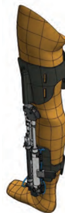
Figure 3: Quasi-passive knee exoskeleton
