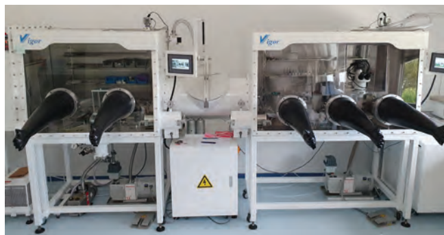
Figure 2: Glovebox system in the Extreme Conditions Chemistry Laboratory
