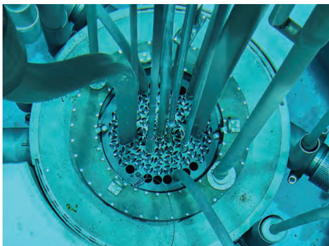
Figure 3: Modified reactor-core configuration.
