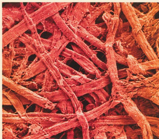
SEM image of paper after oxygen-plasma treatment A Vesel et al 2007 Journal of Physics D: Applied Physics 40 3689–3696
