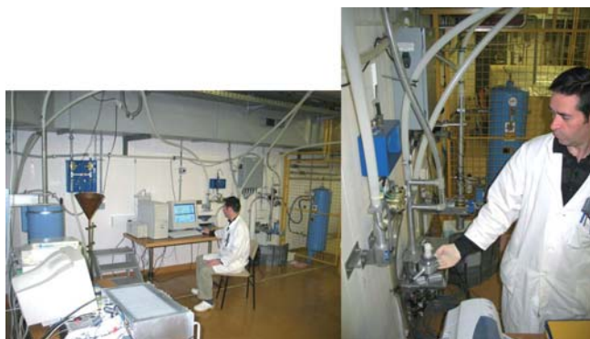
Figure 2: Fast Pneumatic Transfer System (FPTS) with sample transfer time from the reactor core to the HPGe detector of 1 s is used for analyses of short-lived isotopes using INAA method
