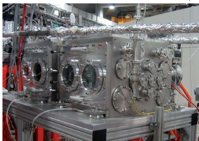
Figure 2: The transmission x-ray microscope Twinmic, developed and installed at the synchrotron light source, Elettra in Trieste in collaboration with seven European partners and the Department of Surface Engineering and Optoelectronics.
