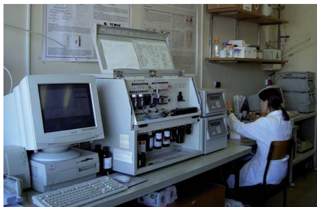
Figure 3: Structural identification of proteins is important part of proteomics. The Edman degradation-based protein sequencer.
