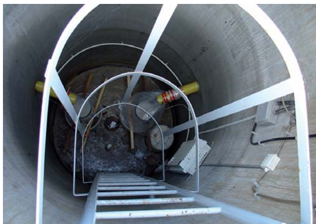
Figure 4: Lysimeter station at an unpolluted meadow at Kleče near Ljubljana: collection of soil water for determination of background levels of pollutants threatening the drinking-water supply for the Ljubljana Municipality
