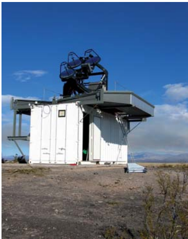
Figure 3: LIDAR station in the Argentinean pampas near Malargue. Our hardware contribution to the Pierre Auger detector uses scattered light from lasers to monitor atmospheric conditions, paramount for proper evaluation of the fluorescence detector data.
