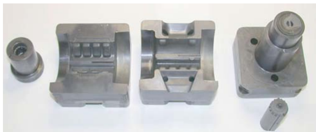
Figure 4: Laser sintered tool for die casting of aluminium alloys protected with TiAlN hard coating.
