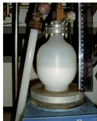
Figure 2: Reaction vessel (700 ml) for the preparation of AlF_3 with high surface area in liquid anhydrous HF
