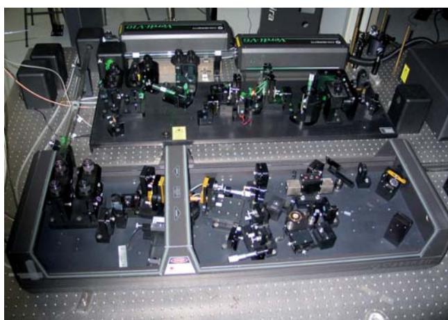
Figure 5: Coherent laser system used as a source of ultra-fast laser pulses shorter than 100fs. It consists of two frequency doubled NdYag lasers (rear of the picture) used for pumping. Laser oscillator (in the middle) uses Kerr-Effect for stable self mode-locked operation giving pulses at high repetition rates, and Regenerative Laser Amplifier (front) amplifies pulses up to a few J per pulse at 300kHz.
