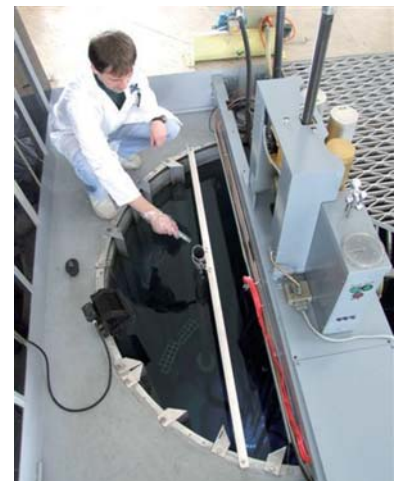
Figure 1: Irradiation of additives for SiC/SiC composite materials developed at the Department for Nanostructured Materials for the first wall of a future fusion reactor.
