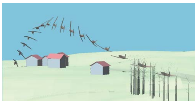
Figure 2. Simulated accident trajectory of the Pilatus PC-9 aircraft following the collision with a tree, at Spodnji Žerjavci, 3 March 2004. View towards west-northwest. R. Krivec; technical report for Ministry of Defence.
