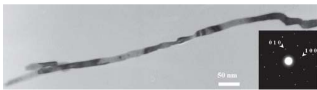
Figure 4: TEM-BF image of KNbO 3 perovskite nano-needle collected along [001] zone axis and the corresponding SAED pattern. Advanced Materials: I. Pribošič, D. Makovec.
