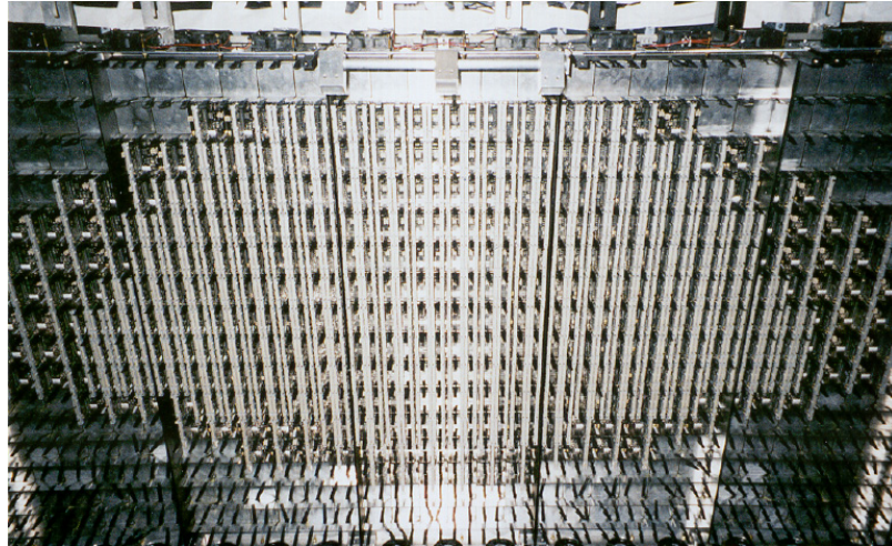
Figure 4.19: Arrangement of the photomultiplier tube base modules on the focal plane of the lower photon detector back plane.
