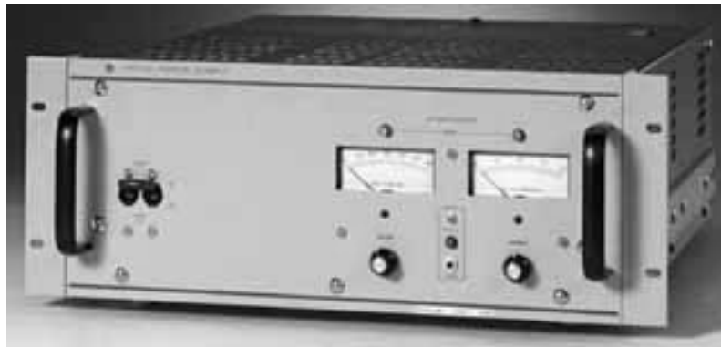
Figure 4.28: Low voltage supply.
